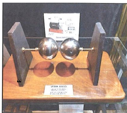
Spark balls similar to this model were used in early wireless transmissions made by Guglielmo Marconi. (1896)
