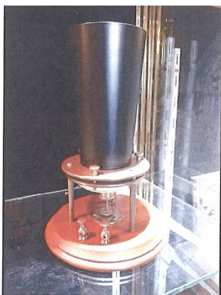
This Liquid Cup Telephone is an accurate reproduction of Alexander Graham Bell's first experimental telephone transmitter of 1876. The first words ever spoken over an electric telephone were "Mr Watson come here I want you".
